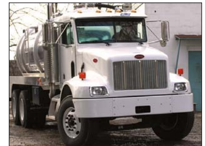
This Peterbilt pumper serves the maintenance side of the business and features a 3,600-gallon aluminum tank from Progress Tank Sales.
